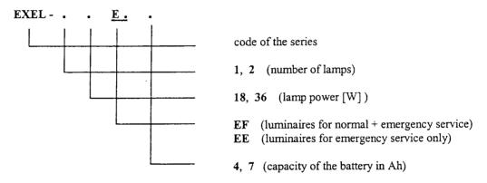
In the luminaires series EXEL the following components can be installed:
