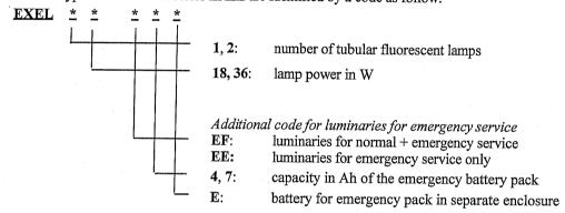
The luminaries EXEL series are suitable for use of tubular fluorescent lamps with G13 bi-pin lampholder.
