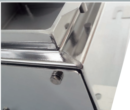
Detail of TIG welding of walls
